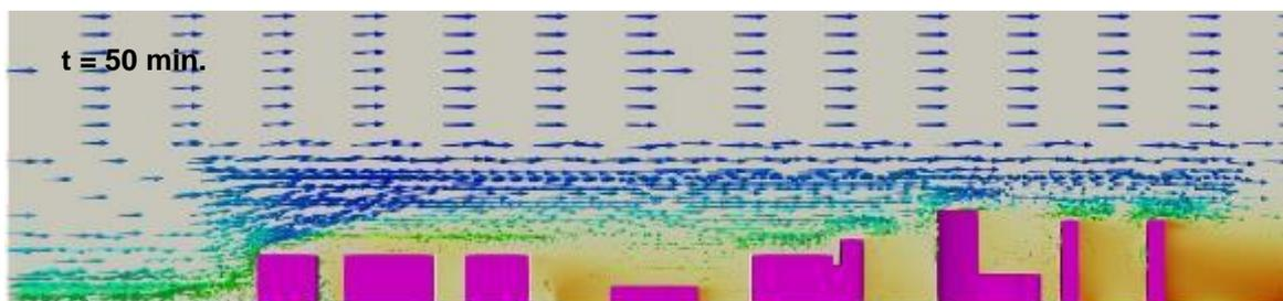
It is confirmed that the high-rise buildings located along the Main Road corridor are slowing down air along the corridor and make it less efficient in transportation of fresh air flowing in from the east. Intensity of air flow along the main air corridors is not constant but varies, depending on the layout of the buildings in the vicinity of the corridors.
