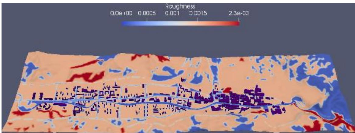
As it was the case in the meso-scale computation, the wall-function approach is used to treat the wall boundaries. The same roughness map, used for the meso-scale case, is also used here, see Figure 7.7. The inflow boundary condition is extracted from the meso-scale computation for the ESE wind direction case for east boundary. The lateral (south and north), top and outflow boundaries are treated as a constant pressure boundary condition.
