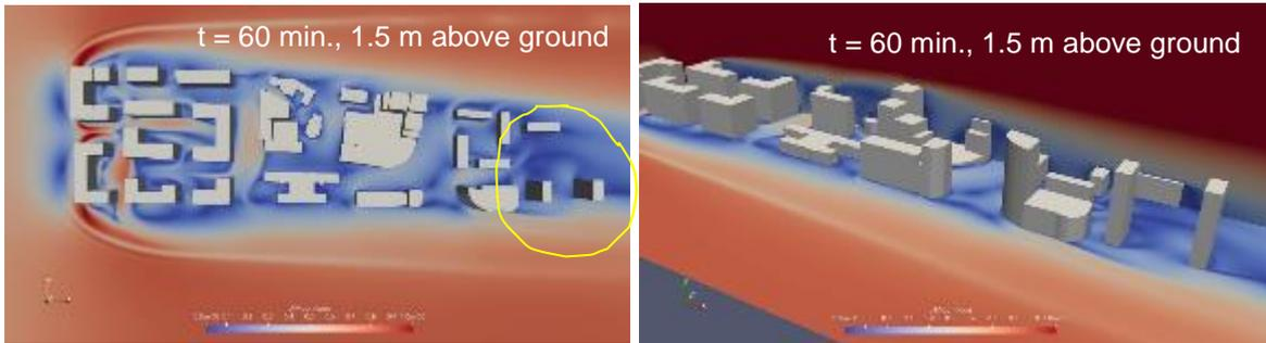
**Figure 9.7 – Top view (left) and side view with cut plane at  $y=102 \text{ m}$  (right) of instantaneous velocity field for custom buildings layout**
