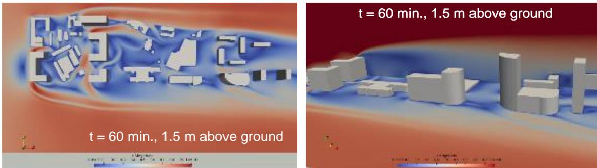
**Figure 9.6 - Top view (left) and side view with cut plane at  $y=102 \text{ m}$  (right) of instantaneous velocity field for regulatory plan buildings layout**
