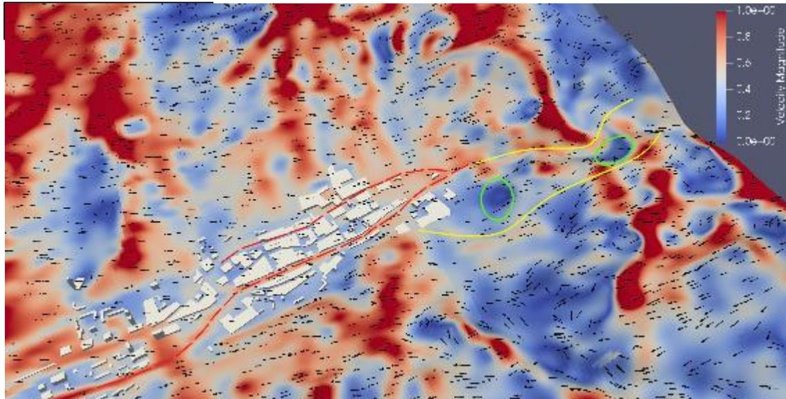
**Figure 8.3: Velocity magnitude field with corresponding vectors for 1.8m/s reference velocity**
