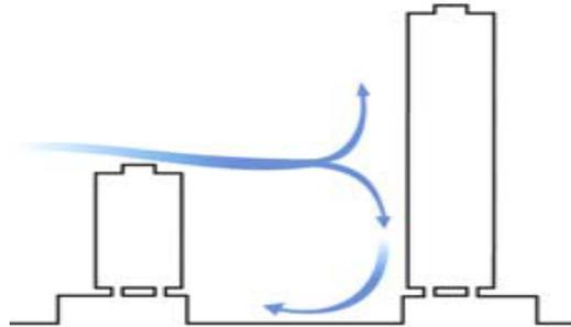
Figure 3.8 - Building height massing showing air circulation [5]
