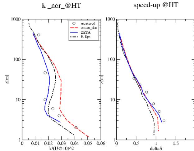
Figure A.5: Vertical profiles of the fractional speed-up ratio ( $\Delta S$ ) (right), and normalised turbulent kinetic energy  $k/U_{10}^2$  (left) at the CP
