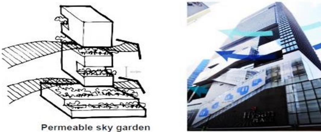
There are a lot of different types of building gaps/openings. For example, one bigger opening can be positioned in the middle of the building. The Kai Tak Development is an example of building which has a characteristic high opening at its centre, through which air flows (Figure 3.11 and 3.12).
