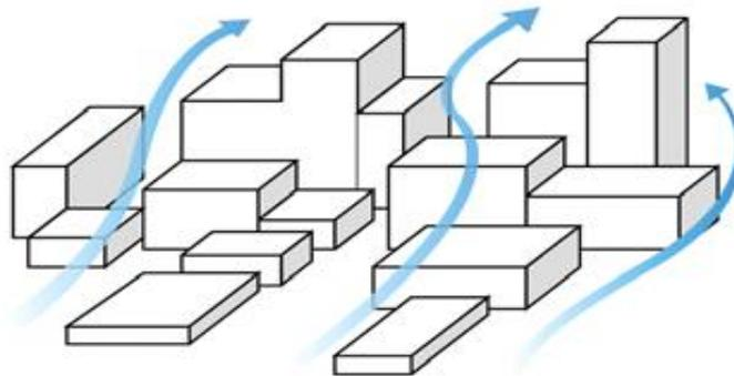
The stepped height concept can help optimise the wind capturing potential of the development itself. A practical example of stepped height buildings is presented in the Kai Tak (Hong Kong) Development Urban Design Guidelines [11]. Difference in height between the first and the second building is approximately 15-20 m, the same as between second and third. The space between buildings has the proportional dimensions and layout to allow air circulation (Figure 3.9).
