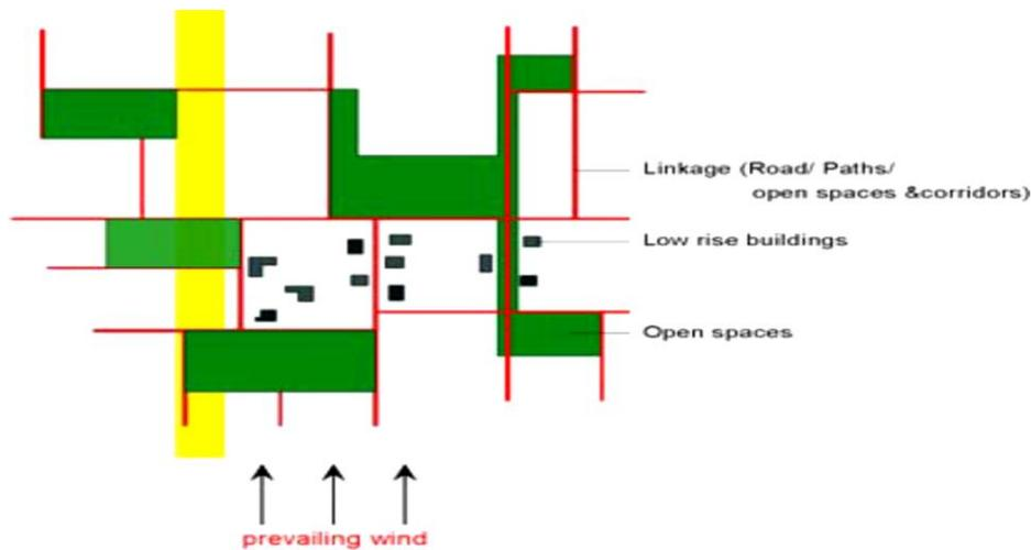
Figure 3.21: Building setback and building permeability, air paths, open spaces (air ventilation connectivity) and greenery [19]
